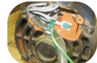
Grounding point in the engine.
