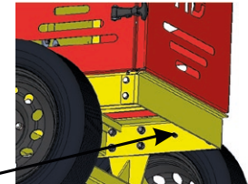
Grounding point in the machine.
