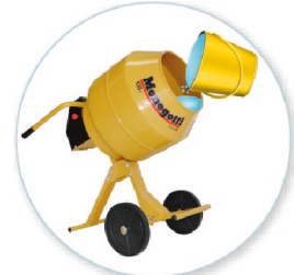
3. Add half of the water and mix for one minute .
