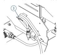
**STEP 03:** Manually adjust the starting point of the water flow on the Water Level valve. Water is only injected into the system in the "forward" direction to ensure wetting only when the dough is in the process of being mixed.
