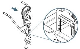
**STEP 02:** Insert the auger into the centre tube, fitting it onto the shaft. Insert the fixing pin (1) and tighten it with a clip (2). If necessary, use a rubber hammer to fit it all the way in.
