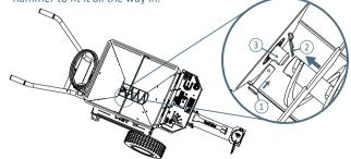
If the shaft is misaligned, plug the machine into the power supply, press the "reverse" button until you are sure that the distributor tube is in the correct position, ensuring the shaft (3) is aligned with the fixing pin (1).
